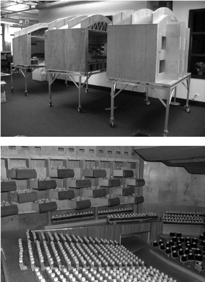
Figure 8.5 Physical model: acoustic model of a concert hall (© Kirkegaard Associates)
