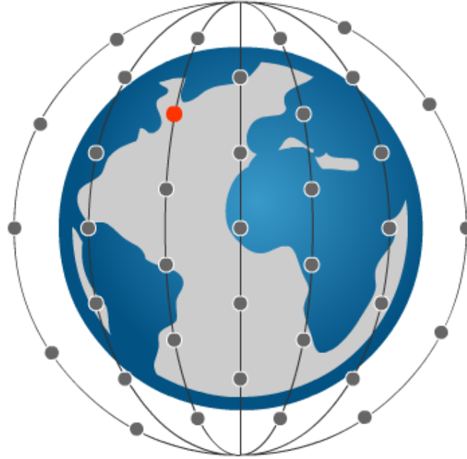
(a) Low earth orbit: Often in polar orbit at 500 to 1500 km altitude
