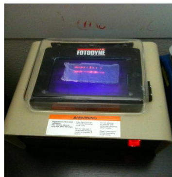
Agarose gel with DNA ladders on a UV transilluminator
