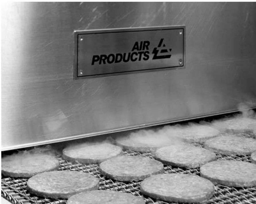
FIGURE 17.4 Examples of cryogenic freezing of foods (Source: 8 1996 Air Products and Chemicals, Inc.; photograph courtesy of Air Products and Chemicals, Inc).
